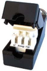
Rear View showing IDC
