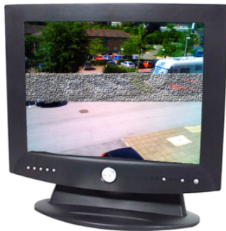
CCTV Image with Hum Bar Problem Due to Multiple Ground Paths or Loops
