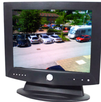
CCTV Image with Ground Loop Isolator to eliminate the Hum Bar
